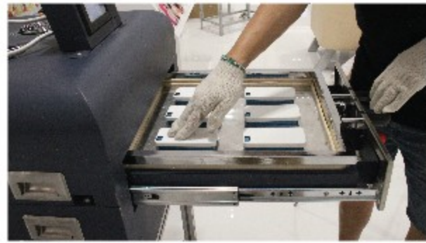
Step 1. Put the phone case on to the printing jig.
