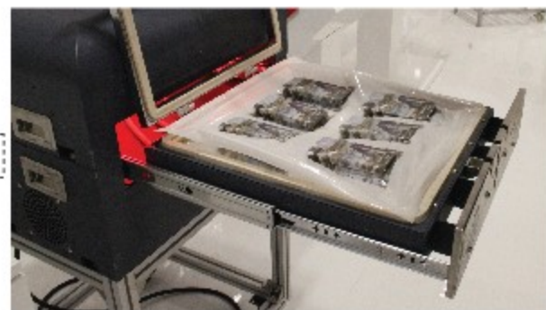
Step 7. Open the positioner then take out the film and the phone cases
