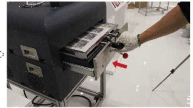
Step 4. Push the platen inside the machine
